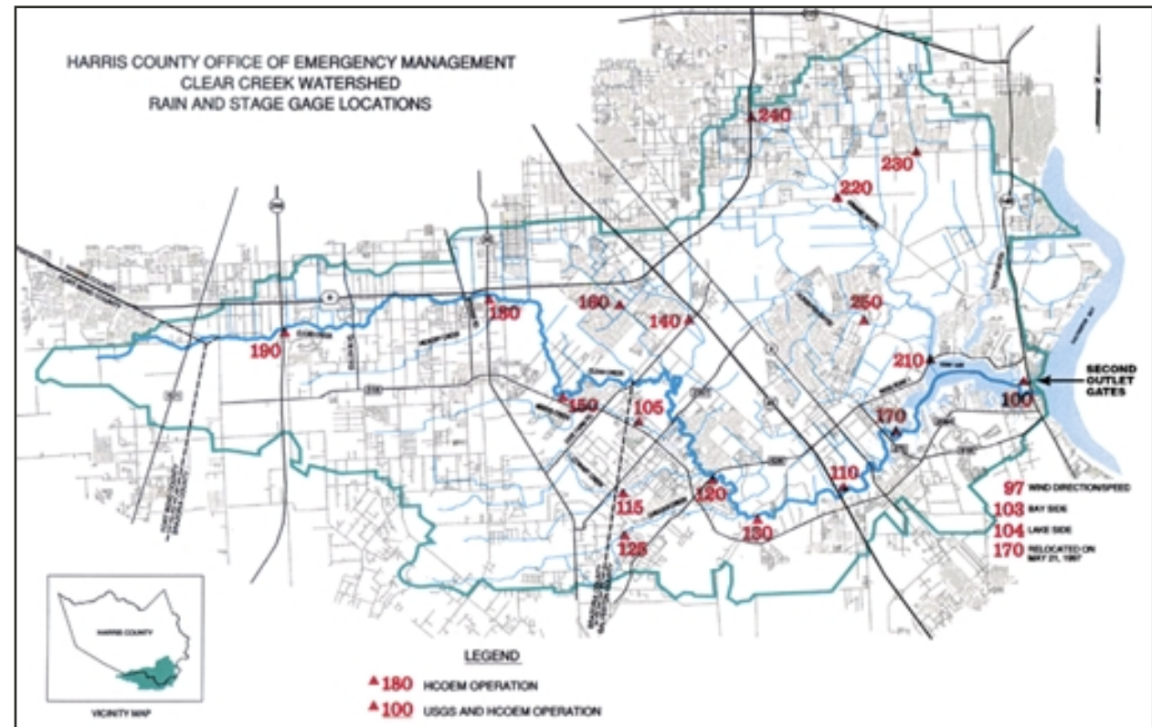
Area map of the Clear Creek watershed and the gage locations for monitoring rain and water levels along Clear Creek, Armand Bayou and other tributaries
